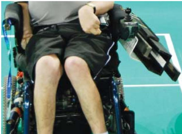
Brackets, baskets and holders attached to the chair are permitted. These can be used to hold equipment off the ground (and keep it from rolling away) and give the player and assistant more room to manoeuvre their chair and ramp inside the playing box.
